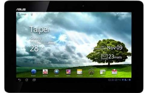
A tablet computer is a combination of the pc and smart phone. They are very portable, typically have a much longer battery life than a laptop computer, have a larger screen than a smart phone. They can connect to the Internet either using wifi (local wireless network) or 3G or 4G (third or fourth generation cellular wireless). Some connect using wifi, some with either wifi or 3G or 4G.
